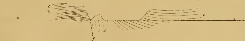
Fig. 10. Sketch section across Singanpur valley. a , Lower Bundair shales with beds of sandstone: b , Red upper Bundair sandstone: c , Grey sandstone: d , Coarse sandstone: e , Sandstone, highest beds of the series: f , Fault.
