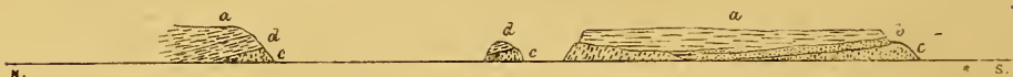
Fig. 5. Section through Gwalior and adjacent hills. a , Kymore sandstone; b , Kymore conglomerate; c , Trap, d , Jasper beds—Gwalior series.
